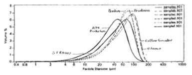
Note: It was assumed that the laboratory ACM-1 could match the ACM production particle size and there it was not run. Comparing the other pieces of equipment it can be seen that the Strand Mill comes close to duplicating an ACM production mill. The following table compares approximate costs, efficiency, ease of cleaning, and particle size for each unit.
